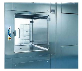
Pass Box PiBi is designed accurately, with the lowest number of joints and with all the internal surfaces round-cornered. It is manufactured in stainless steel AISI 304 Scotch Brite finishing (stainless steel AISI 316 as option), glass doors with tight gaskets, external hinges and stainless steel handle.
