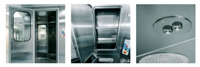
This solution helps to prevent any propagation of dangerous particles outside the isolated area and allows the worker to remove contaminated clothing and avoid breathing in potential harmful substances. The best strategy to achieve this purpose is to saturate quickly the area inside the shower, spraying water drops of 5-10  $\mu$  to wet the surfaces and create droplets on the clothing.
