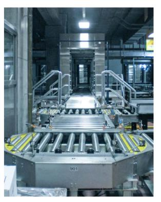
Material handling systems are manufactured in stainless steel AISI 304 or 316, both structure (frames, covers) and mechanics (rollers, chains, sprockets).
